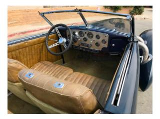
The interior is also patterned after a Cord, including pleated leather front seats, rear seats, and door panels. The windshield was re-chromed, assembled, and installed during the refurbishment. The deteriorated top frame and cover are useful only as patterns, though an original oval rear window was included.
